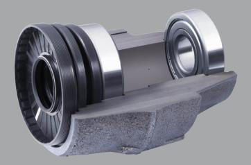
Encore washers are built with **two commercial grade SKF bearings**. These premium bearings are sealed for maximum protection leading to longer life with fewer repairs. The three individual seals with 5 lips provide a water-tight barrier around the drive shaft to protect the bearings from damaging moisture. To ensure better performance, the durable AC motor has no brushes.
